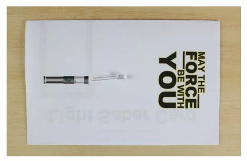
Fold the template and insert the LED legs thru the holes. Note that one leg goes in each cut.
