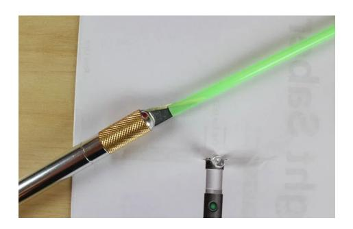
Take the Xacto or scissors and slice 1/4" on one edge of the straw. This is so the straw will fit over the LED. If the straw already fits then this step isn't necessary.
