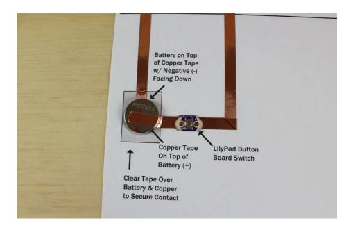
Once the battery and switch are in place, use transparent tape to secure them over. Make sure the switch and battery are contacting the copper tape firmly.
