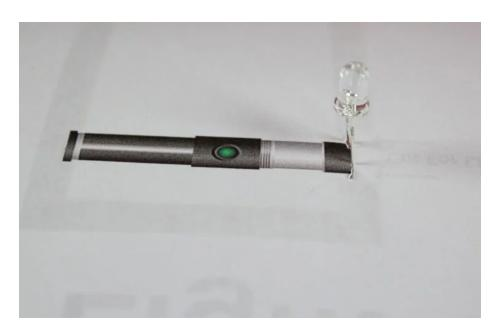
Once the LED has been put thru the cuts, flip the template over and bend the legs so that they contact the copper tape. Again, make sure the positive LED leg is touching the positive side of the copper.
