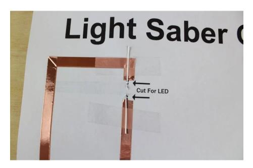
Once everything is in place you can tape down the legs with transparent tape. Make sure the legs are making firm contact with copper.
